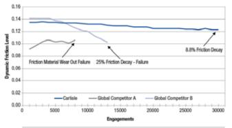
Glazing / Fade Resistance Under Heavy Braking Carlisle offers superior resistance to glazing verses competitive materials.
